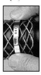
4. Attach the hoist line to the Hoisting Grip as shown. Apply tension slowly to the hoist line, allowing the Hoisting Grip(s) to tighten uniformly on the cable.
