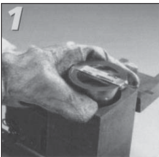
1 Insert CADWELD PLUS package into mold (optional: use with or without cover/baffle)
