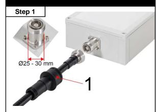
RJB (1) comes preassembled on the jumper cable. It is designed to seal to the smooth neck of the standard 7-16 DIN female bulkhead with an OD of 25–30mm.
