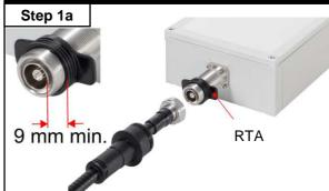
Install the Rosenberger Thread Adapter (RTA), p/n SLWK112-C03/51 (sold separately) in the correct position per the photo above (9mm from front connector interface). There must be adequate thread length to provide this 9mm and space for the RTA. The RTA is required to achieve IP68 sealing with the RJB to the fully threaded version of the 7-16 DIN bulkhead. Please proceed to step 2.
