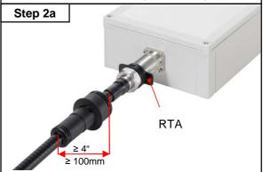
Turn the RTA counterclockwise until it comes in contact with the DIN connector nut. Verify the RTA is squarely aligned with the connector nut and seated into the bulkhead threads. Please proceed to step 3A.
