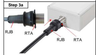
In this installation, the RJB lands on the RTA as shown in the inset photo above, providing IP68 sealing. The RJB must be installed squarely to the RTA with no more than 1 of the 3 RTA grooves exposed. The 2 RTA tabs will be exposed, providing visual proof of proper installation. Do not squeeze the circumference of the RJB after installation as this can cause future water ingress.
