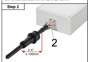
Straighten the cable  $\geq 4$  inches (100mm) from where it exits the 7-16 DIN male connector. Ensure cable and connector are clean. Connect the jumper cable to the device and properly torque the connection.
