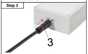
Slide the RJB until it stops across the connection. Final position according to the inset photo above. RJB lands on the smooth diameter beyond the threads of the female connector, providing IP68 sealing. Do not squeeze the circumference of the RJB after installation as this can cause future water ingress.
