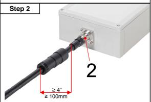
Straighten the cable ≥ 4 inches (100mm) from where it exits the 4.3-10 DIN male connector. Ensure cable and connector are clean. Connect the jumper cable to the device and properly torque the connection.
