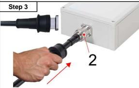
Slide the RJB until it stops across the connection. Final position according to the inset photo above. RJB lands on the smooth diameter beyond the threads of the female connector, providing IP68 sealing. Do not squeeze the circumference of the RJB after installation as this can cause future water ingress.
